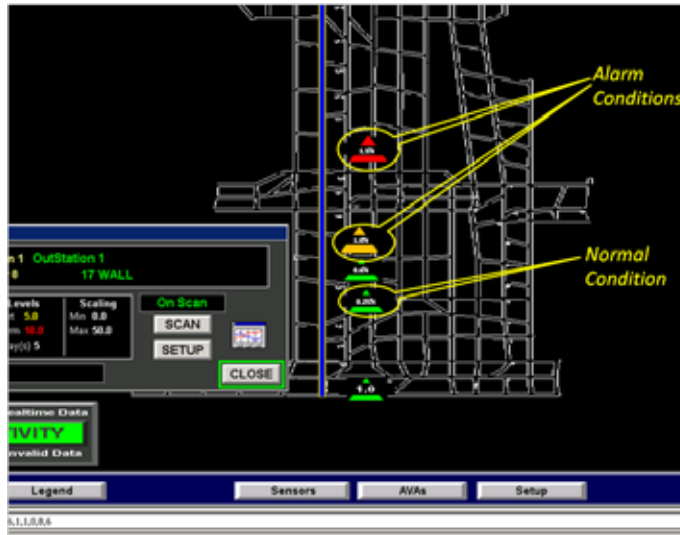
Example of data display on a MSHA approved Atmospheric Monitoring System.
