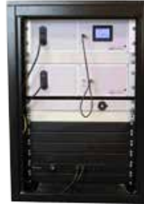
Example of Central Control Unit placed outside of explosive area.
