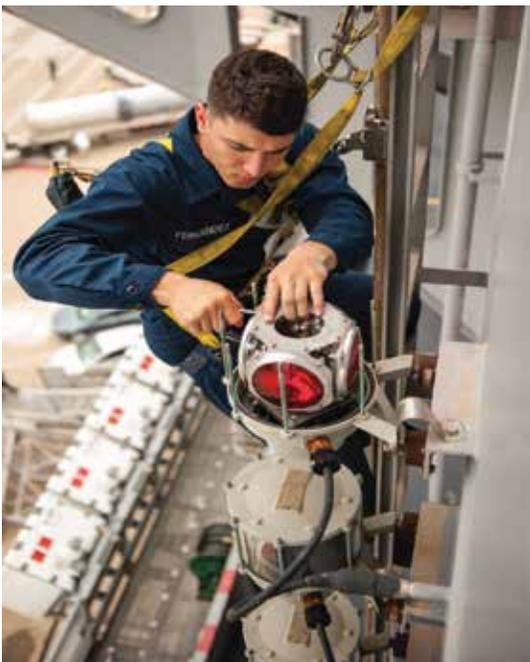
**Above:** RSL luminaires can be provided with a non-metallic adapter base to fit into the legacy lights' footprint, eliminating the need for hot work during retrofits and upgrades.
